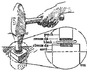
Fig. 3: Diagram of hand minting showing the shock absorption effect of the planchet ("blank").<sup>4</sup>
