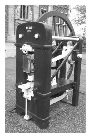
Fig. 2: Coin press formerly used at the Utrecht Mint (Netherlands).<sup>3</sup> The coin dies have been removed, but it can be seen that the lower die was set in a plate in the immobile base, while the upper die was attached to the rocker arm.
